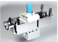
6.Match with the KEY and align the cap with IDC until it clicks as shown. press the cap down to IDC.
